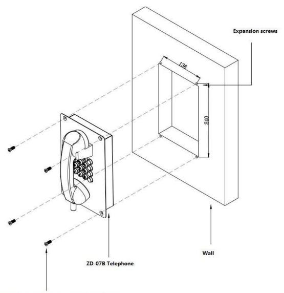
4-M5\*20Cross countersunk head machine screw
